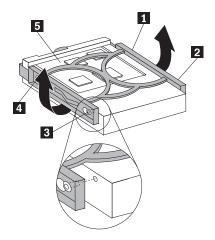
Figure 22. Installing the primary hard disk drive into the bracket
